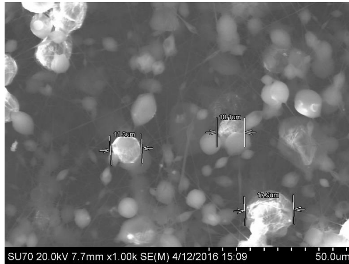
Figure 57 Nano mesh showing beads at 1K magnification
