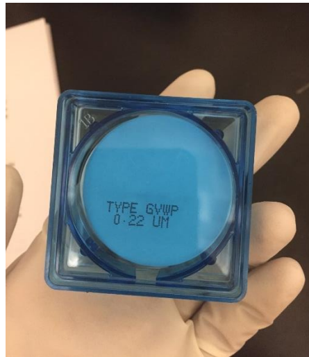
Figure 45 GVWP durapore membrane with pore size 0.22 \mu\text{m}
